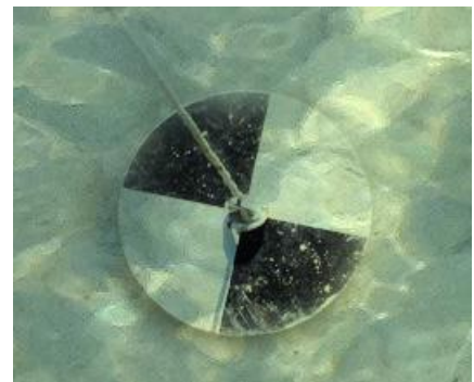
A significant decreasing trend in water clarity has been documented in Great Pond over the past 10 years as measured using a Secchi disk.
